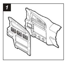
Disconnect the negative battery terminal to prevent an accidental short circuit. Unclip the entire dash trim bezel. Remove the screws securing the factory head unit and disconnect the wiring.
